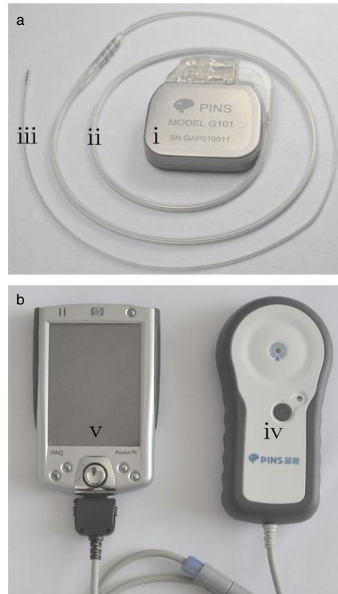
**Figure 1.** Photo of PINS device. a. implantable parts including (i) implantable pulse generator (IPG), (ii) extension, and (iii) lead; b. telemetry/programming parts including (iv) controller and (v) personal digital assistant (PDA).
